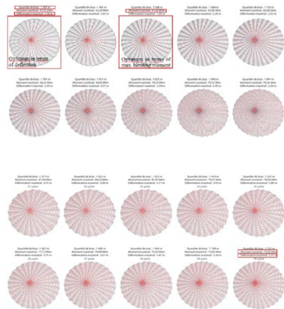
Top: Deflection and bending moment measured on a variation on the shifting - Bottom: and on the number of wedges - data extracted from Karamba3D model
