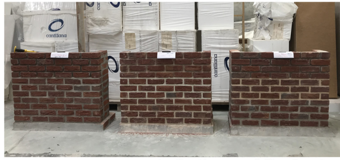
testing the reversibility of mortars
