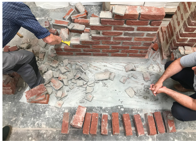
testing the reversibility of mortars
